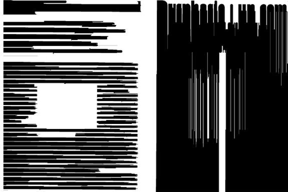
(a) Original document image (b) After horizontal smearing (c) After vertical smearing
