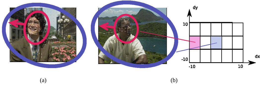
Fig. 4: Two interview scenes showing a typical motion pattern, and a spatiogram over motion vectors in [-10, 10] \times [-10, 10] capturing this information.
