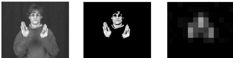
Fig. 2. Example of the features used by the classifier: original image (left), thresholded image (center), and down-scaled image (right)
