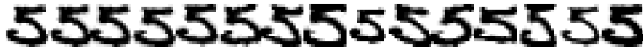
Fig. 2. Example of first-order approximation of affine transformations and line thickness. (Left to right: original image, \pm horizontal translation, \pm vertical translation, \pm rotation, \pm scale, \pm axis deformation, \pm diagonal deformation, \pm line thickness)
