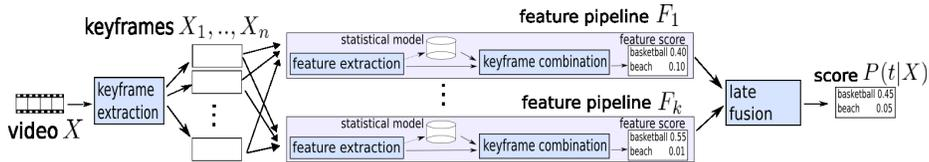
**Fig. 2:** An overview of our tagging system: a video  $X$  is represented by keyframes  $X_1, \dots, X_n$ . Each of them is fed to feature pipelines  $F_1, \dots, F_k$ , in which visual features are extracted and give scores  $P_{F_j}(X_i)$  for each keyframe. These posteriors are fused over all keyframes, and finally over all features, to obtain the result  $P(t|X)$ .
