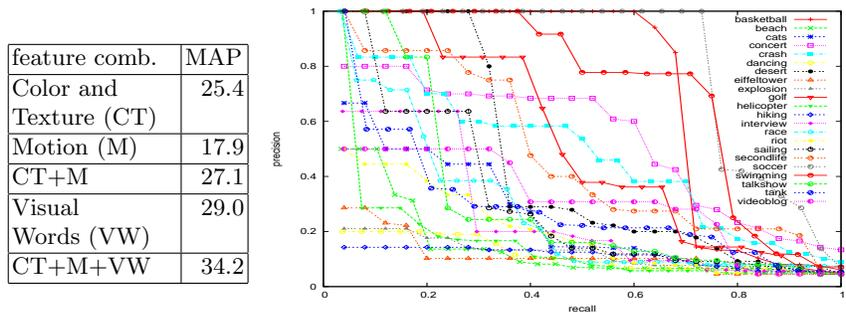
**Fig. 4:** **Left:** Experimental results for several feature combinations in terms of mean average precision (MAP). **Right:** The recall-precision curves when fusing all features. The average precision per concept varies between 81% (`soccer`) and 11% (`hiking`).
